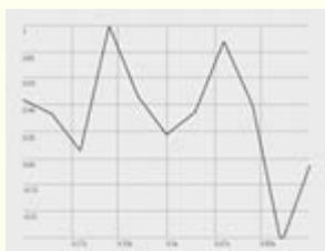
Sine-noise (producing random sinusoidal ramps at the defined frequency)
