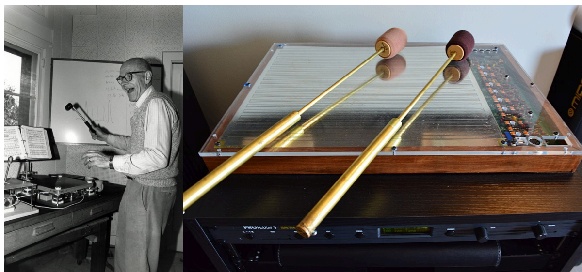
Figure 3.12. Radio Drum and Radio Baton . Right: Max Mathews playing an early version of the Radio Drum around 1984 (Park & Mathews 2009). Left: A recent version of the Radio Baton connected to an E-Mu Proteus 1 MIDI-controlled sound module below it (photo by Daniel Hartwig, Wikimedia Commons).
