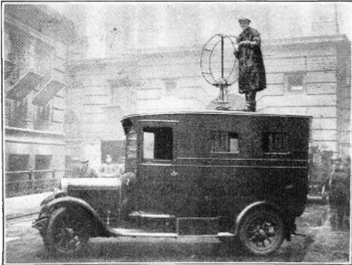
Figure 2.29. Interference-tracking lorry with manually operated directional loop antenna used by the British Post Office to locate unlicensed amateur transmissions and self-oscillating radio sets, 1927 (public domain, Wikimedia Commons).
