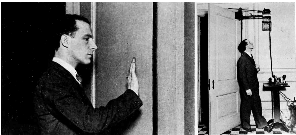
Figure 3.7. Theremin demonstrating a capacitive sensing system designed for opening doors with a wave of the hand, based on the same technology as his instruments (from “ Electrons in new industrial miracles ”, 1932).
