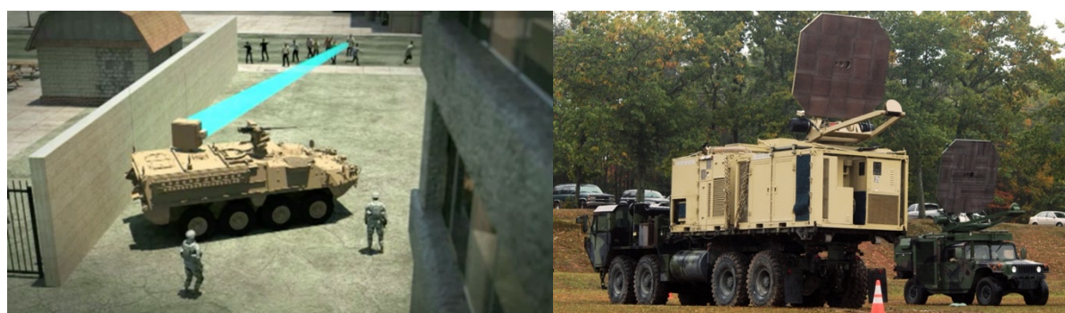
Figure 5.27. The Active Denial System , a microwave-based weapon promoted as a 'safe' and 'non-lethal' crowd control alternative, created by Raytheon and deployed by the US military. Left: a mockup from a promotional video (still from Fogel, 2013). Right: Photo of the operational system from a media event by the US Marines (from https://commons.wikimedia.org/w/index.php?curid=23146873.jpeg ).
