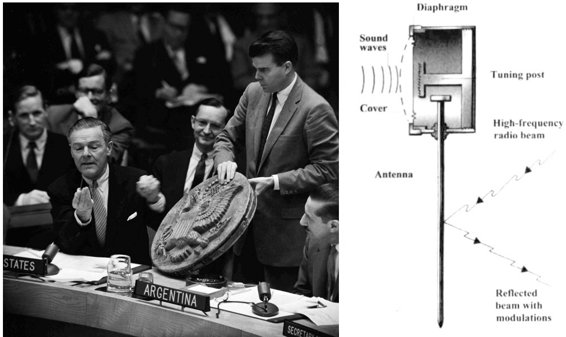
Figure 3.8. Termen's Great Seal bug . Left: a replica demonstrated in front of the UN Security Council by the US Ambassador to the United Nations, Henry Cabot Lodge Jr, in May 26 th , 1960. Smiling behind him is the Soviet Minister of Foreign Affairs, Andrey Gromyko (Photo by John Rooney, AP). Right: a schematic of the mechanism and the basis of its operation (from Melton, 1996).
