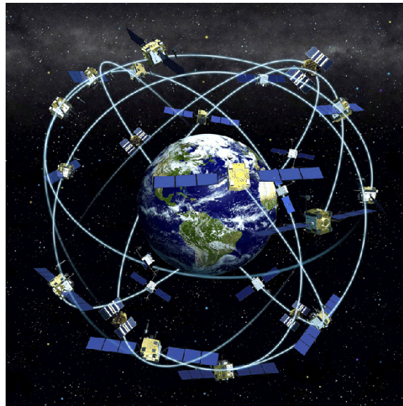
Figure 5.4. A graphic depiction of the GPS constellation of satellites surrounding the Earth. There are at least 4 satellites visible from any point on the planet (Public Domain image by NOAA, https://commons.wikimedia.org/w/index.php?curid=4118967 ).
