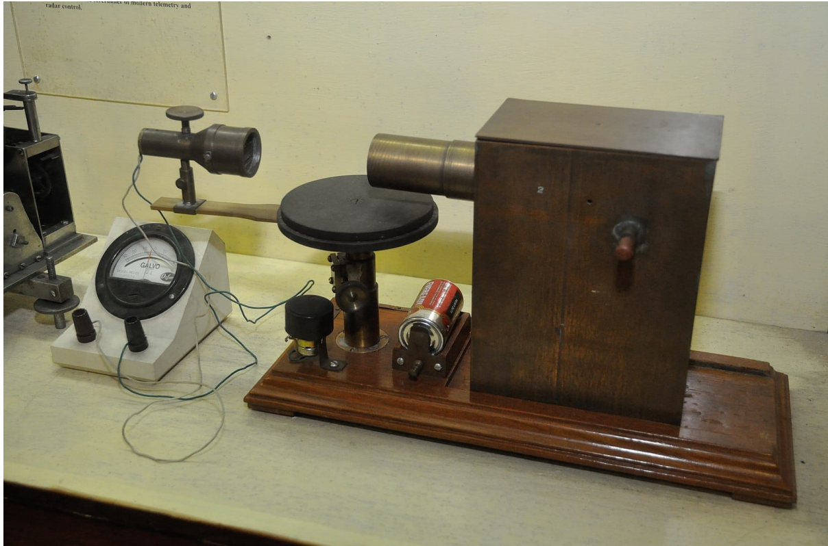
Figure 2.18. Photo of the 60GHz microwave transmitter and receiver devices invented by J. C. Bose and used in his innovative experiments in 1897. The box on the right contains a spark gap transmitter and is made of metal to shield its coil, preventing its EMF noise to reach the receiver; its microwave transmissions radiate via a tubular waveguide. The receiver is on the left and also uses a tubular horn antenna with a galena point crystal rectifier in it and a galvanometer to display wave detection. All equipment pictured is original, besides the battery and galvanometer (photo by Biswarup Ganguly, Wikimedia Commons).
