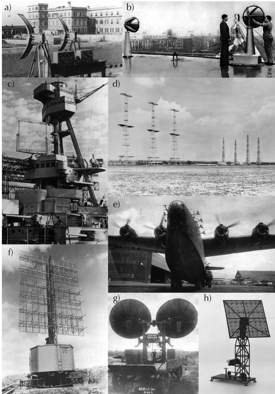
Figure 2.41. Photos of various early radar systems invented in the 1930s-40s in different countries: (a) Italy: Radio Detector Telemetro being tested on a terrace in Livorno in 1936 (Galati 2014); (b) France: Maurice Ponte and Henri Gutton testing their radar on board an ocean-liner in New York in 1935 (Blanchard 2010); (c) US: a battleship with the XAF radar antenna visible from late 1938/early 1939 (National Museum of the U.S. Navy, Wikimedia Commons); (d) Great Britain: Chain Home radar installation in Sussex in 1945, with a line of three remaining transmitter towers on the left (originally four) and a transmitter building in front of them, and a rhombus of four receiving towers in the right, with the receiving building between (Royal Air Force photographer, Wikimedia Commons); (e) Japan: H-6 radar system (in service since 1942) installed on a Kawanishi H8K2 aircraft, with two frontal Yagi antennas and a pair of dipoles on each side of its nose (date of photo unknown, www.worldwarphotos.info ); (f) Germany: Freya radar (date of photo unknown, U.S. National Archives and Records Administration, Wikimedia Commons); (g) USSR: Burya , a mobile aircraft detection unit with dual parabolic antennas (date of photo unknown, Yanovsky 2016); (h) Netherlands: scale model of von Weiler's 'electric listening device' (Museum Waalsdorp).
