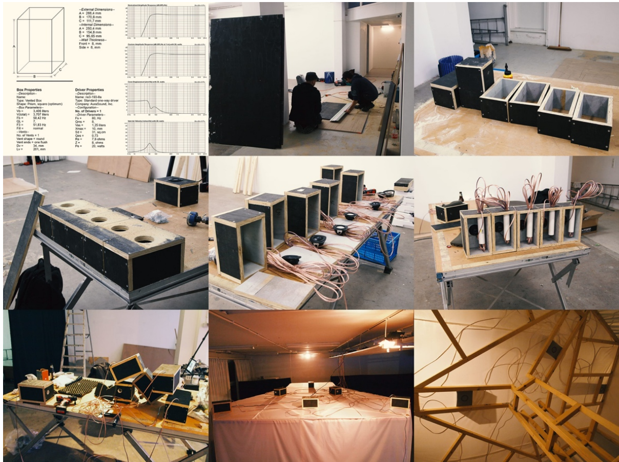
Figure 7.44. Images of the fabrication process of the embedded speakers for The Water Within (Hertzian Field #3) during Modern Body Festival 2016 : From schematics, to building their cabins from leftover plywood, to adding drivers and cables, to mounting them to the structure.
